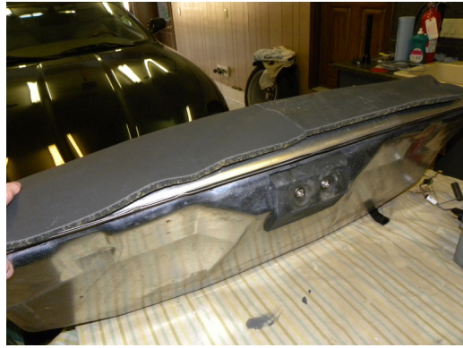
View of front side of tank (shows connection point of the two fuel lines).
