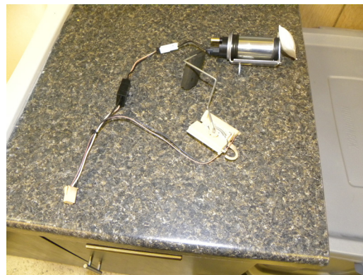
New fuel pump, level sensor and harness.
