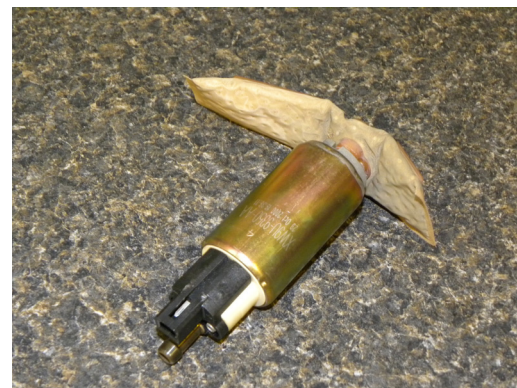
Old fuel pump, bracket removed.
