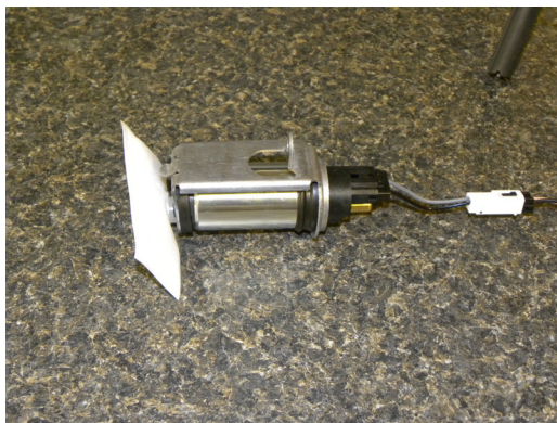
New fuel pump with filter and harness.
