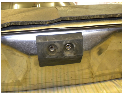
Close up of front side of fuel tank (connection point for two fuel lines).
