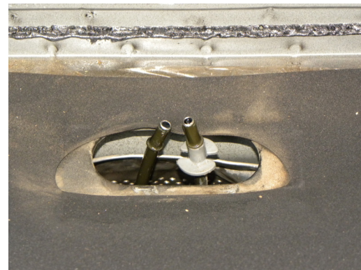
Close up showing the two fuel lines entering trunk. One has removal tool on it.
