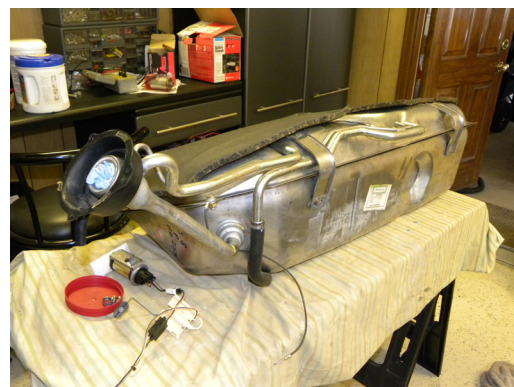
Fuel tank with fuel pump & sensor ready to install in tank.
