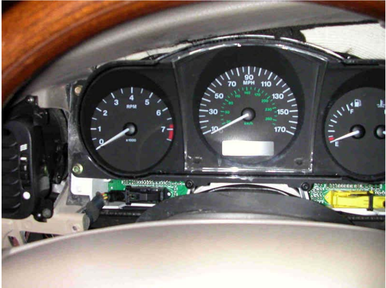
This view shows the instrument cluster out of the car.
