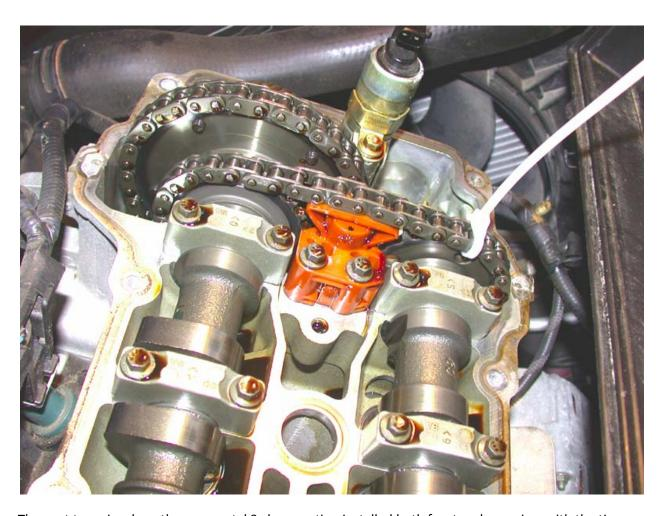
The next two pics show the new metal 3rd generation installed both front and rear view with the tie wrap still installed. Don't forget to remove the tie wrap.
