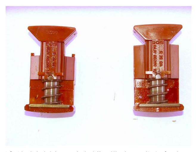
At first I thought they looked pretty good and probably would have kept on cooking. But after a close look as you get in the last picture cracks were starting just above the notch cut out at the bottom of the barrel. As you can see in the picture the cut out has sharp corners that cause stress concentration in that area which in turn causes fatigue cracking.
