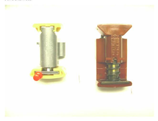
The next picture shows the two removed plastic tensioners.
